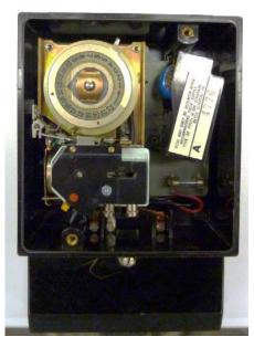
Figure 3.5: Photograph of K22 Receiving Relay with and without Cover
